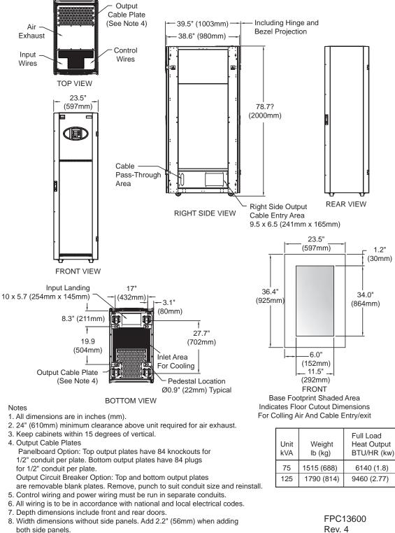
9. Clearance of 36" (914mm) minimum is recommended at front and rear for service access.
