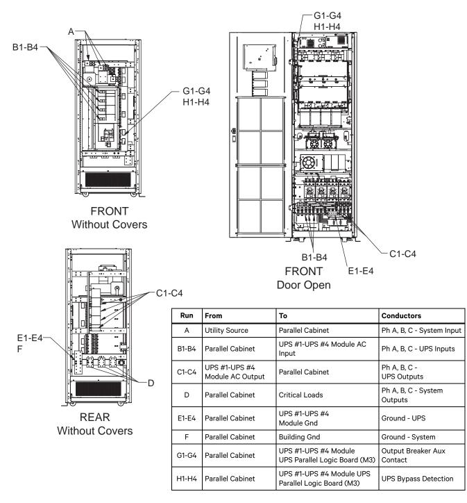
Figure 48 Liebert NX 480V 40-120kVA UPS to Paralleling Cabinet Interconnection—Configuration BB0, FB0, KB0 parallel connection to Liebert NX
