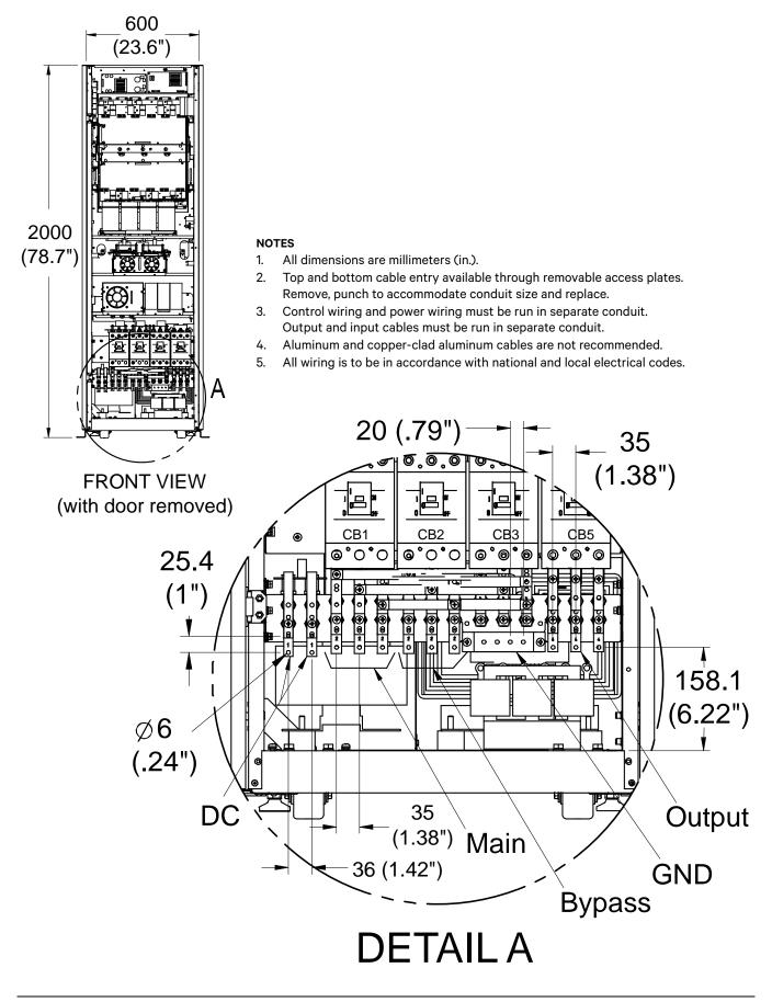
Figure 36 Liebert NX 160-200kVA cable connections
