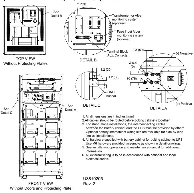
Figure 38 Terminal details, 33" battery power pack system, single cabinet Liebert NX
