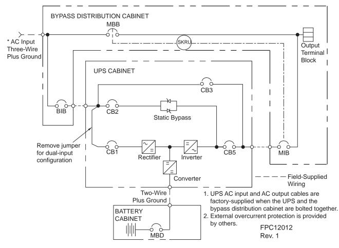
Figure 21 Single-input UPS with external Liebert BDC without internal transformer—typical configuration
