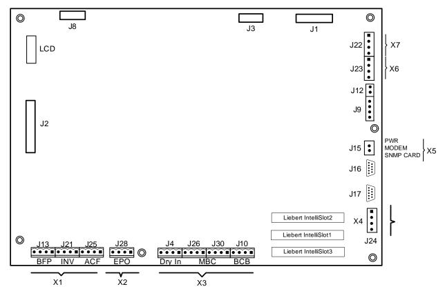
Figure 5 Auxiliary terminal block detail (Monitoring Board)
