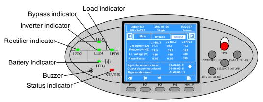
The current operational status of the Liebert NX is indicated by the color of the indicators—green, amber or red—and whether they are ON (solid), flashing or OFF. **Table 27** provides a guide to interpreting the various states of the indicators.
