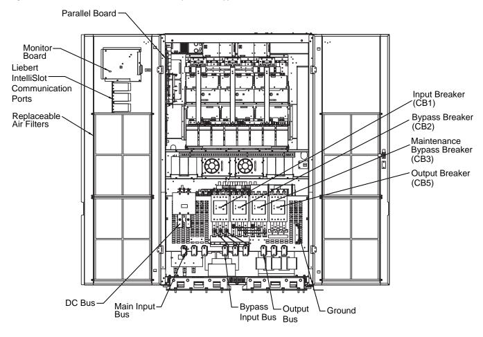
Figure 34 Liebert NX 160-200kVA main components—typical unit
