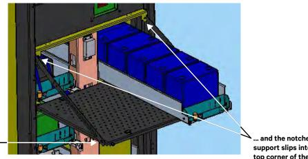
Slot in the support is secured by a screw-in connector at the corner of the battery tray... ... and the notched end of the support slips into the slot at top corner of the battery compartment.
