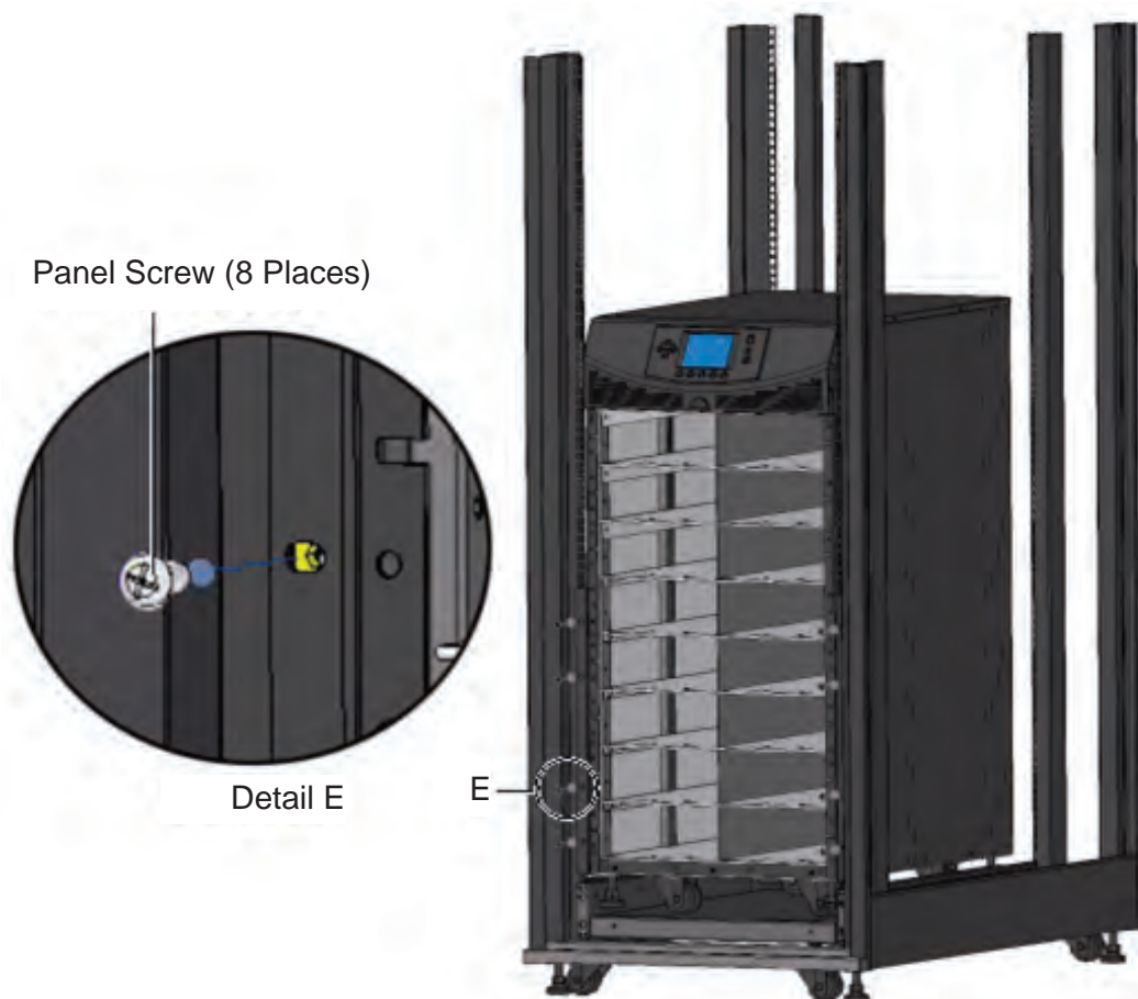
Figure 23 Fix the UPS frame
