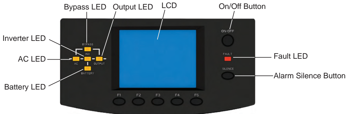
Figure 52 User interface module layout
