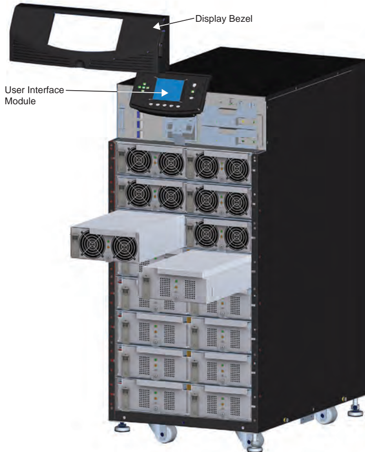
Figure 73 Replacing the user interface module
