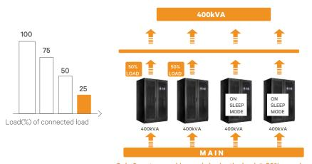
Only 2 system working and sharingthe load @ 50% ensuring highest efficiency operating band
