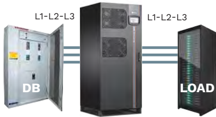
3-wire (L1-L2-L3) installation
