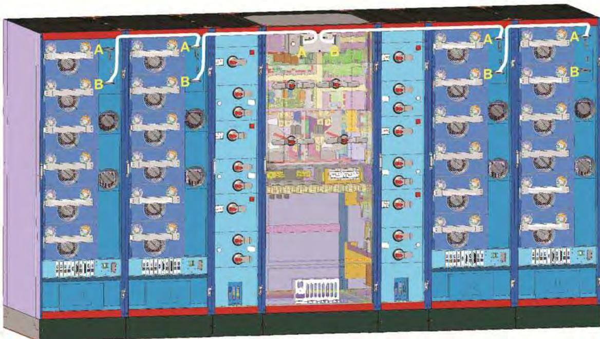
Picture 53 – Connecting the bus cable
