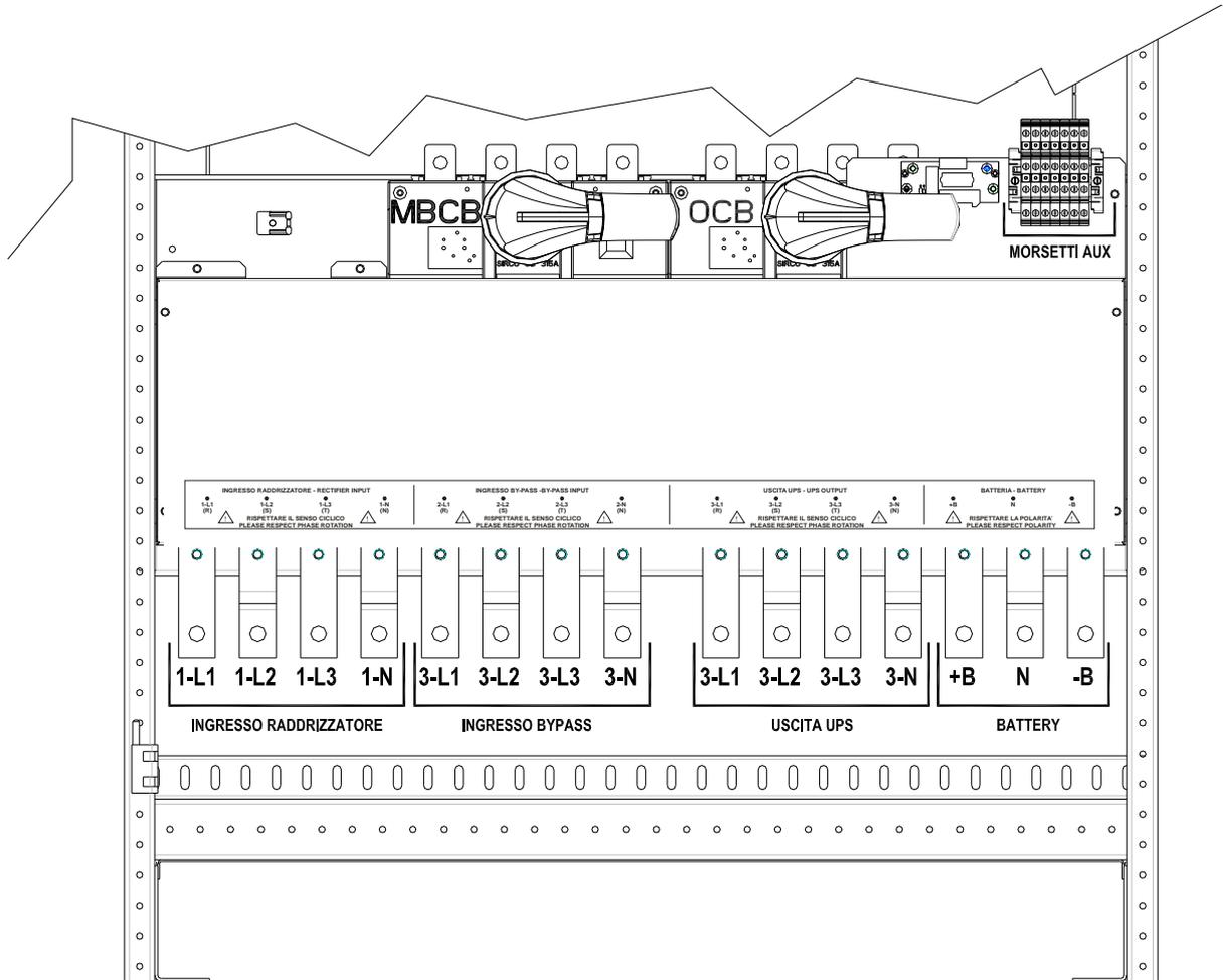
Figura 6 – Morsettiere KEOR HPE200 kVA
