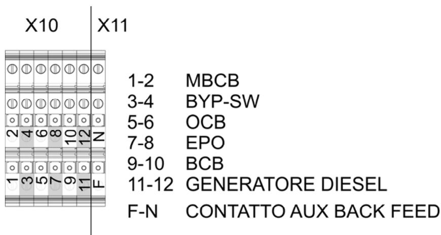
Figura 7 – Morsetti ausiliari KEOR HPE 200 kVA
