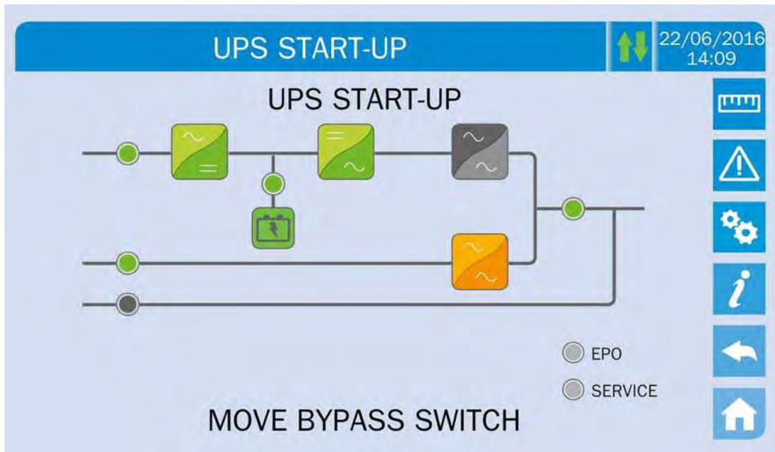
Picture 23 – Transferring the load
