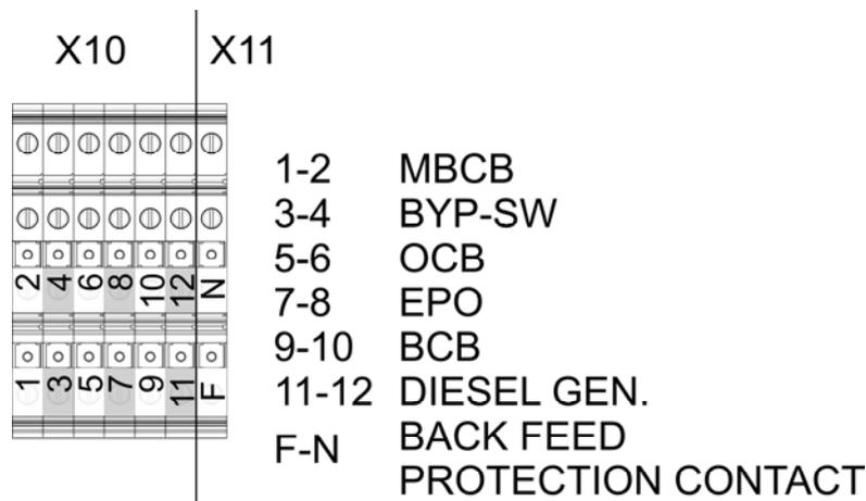
Picture 7 – Auxiliary terminals of KEOR HPE 200 kVA
