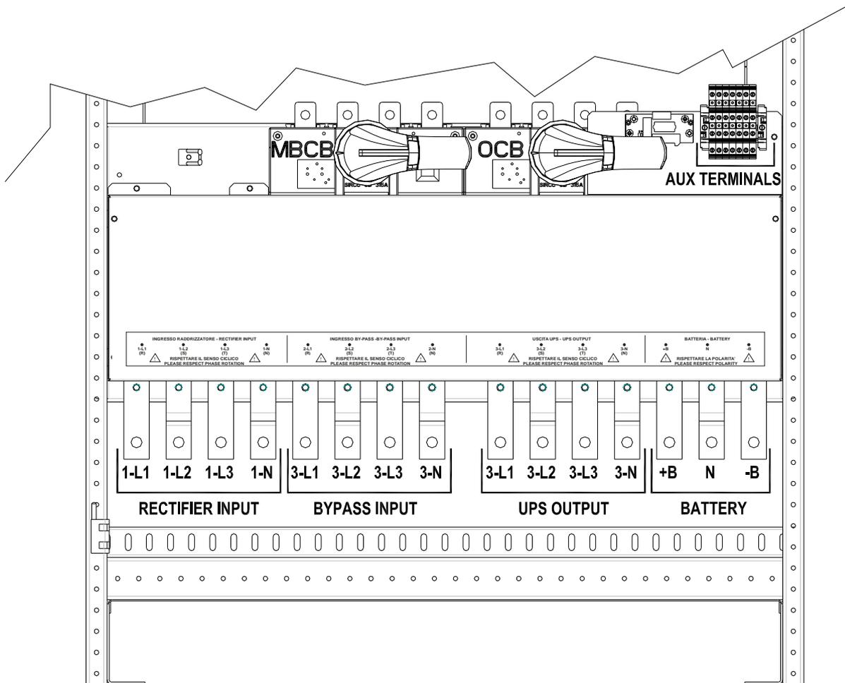
Picture 6 – Terminal board KEOR HPE 200 kVA
