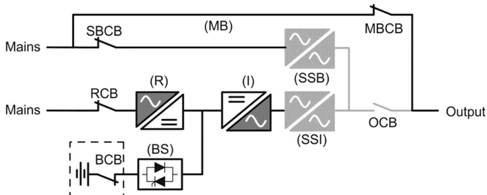
Picture 6 – Manual bypass for functional checks
