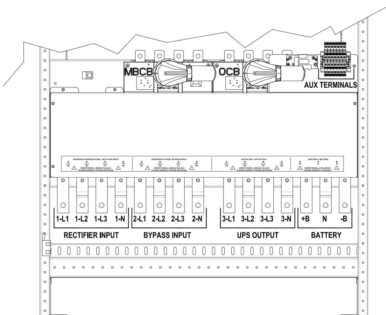
Picture 6A – Terminal board KEOR HPE 300 kVA
