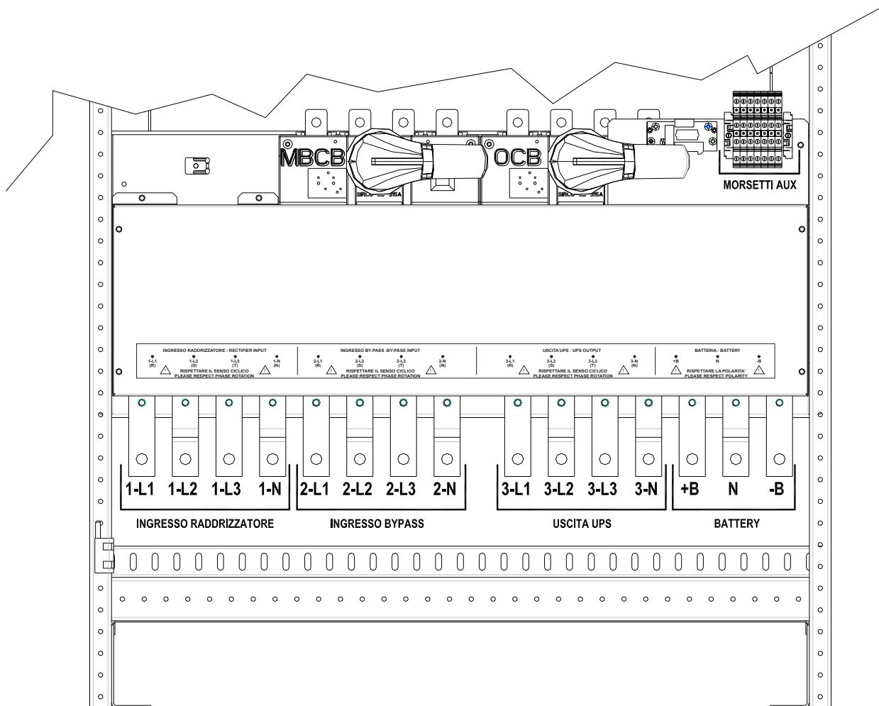
Figura 6 – Morsettiera KEOR HPE 200-250 kVA
