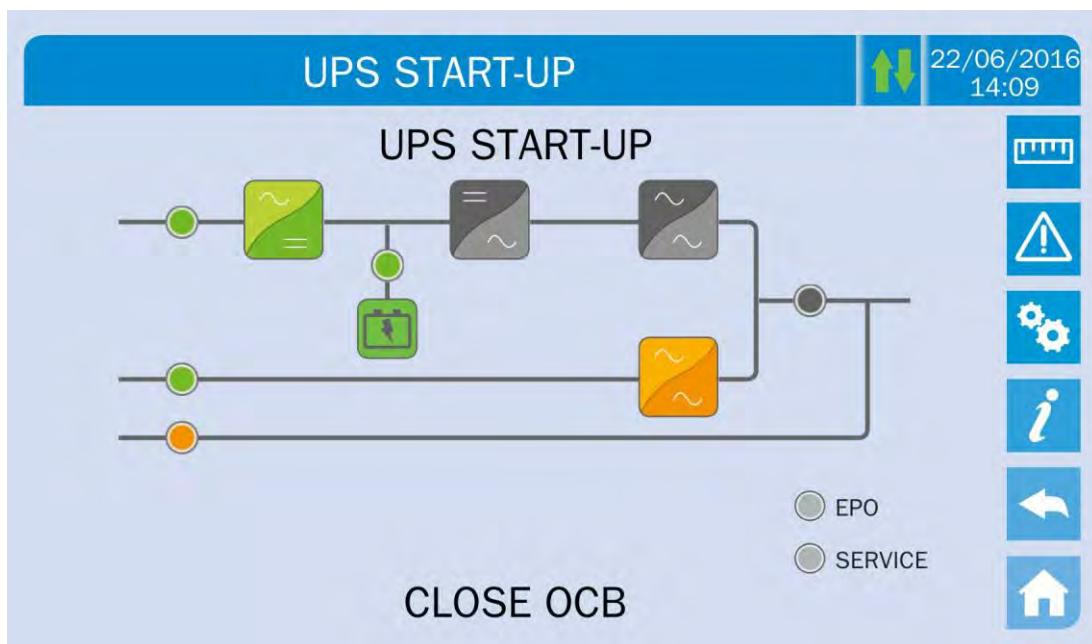
Picture 20 – Closing the UPS output switch
