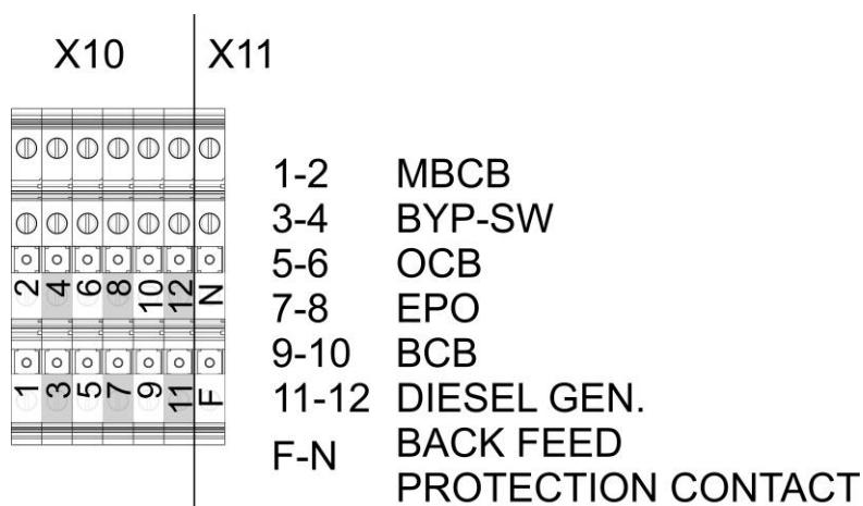
Picture 7 – Auxiliary terminals of KEOR HPE 200-250-300 kVA
