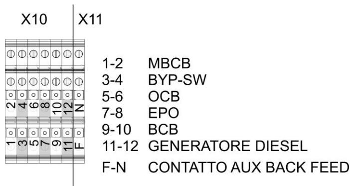
Figura 7 – Morsetti ausiliari KEOR HPE 200-250-300 kVA
