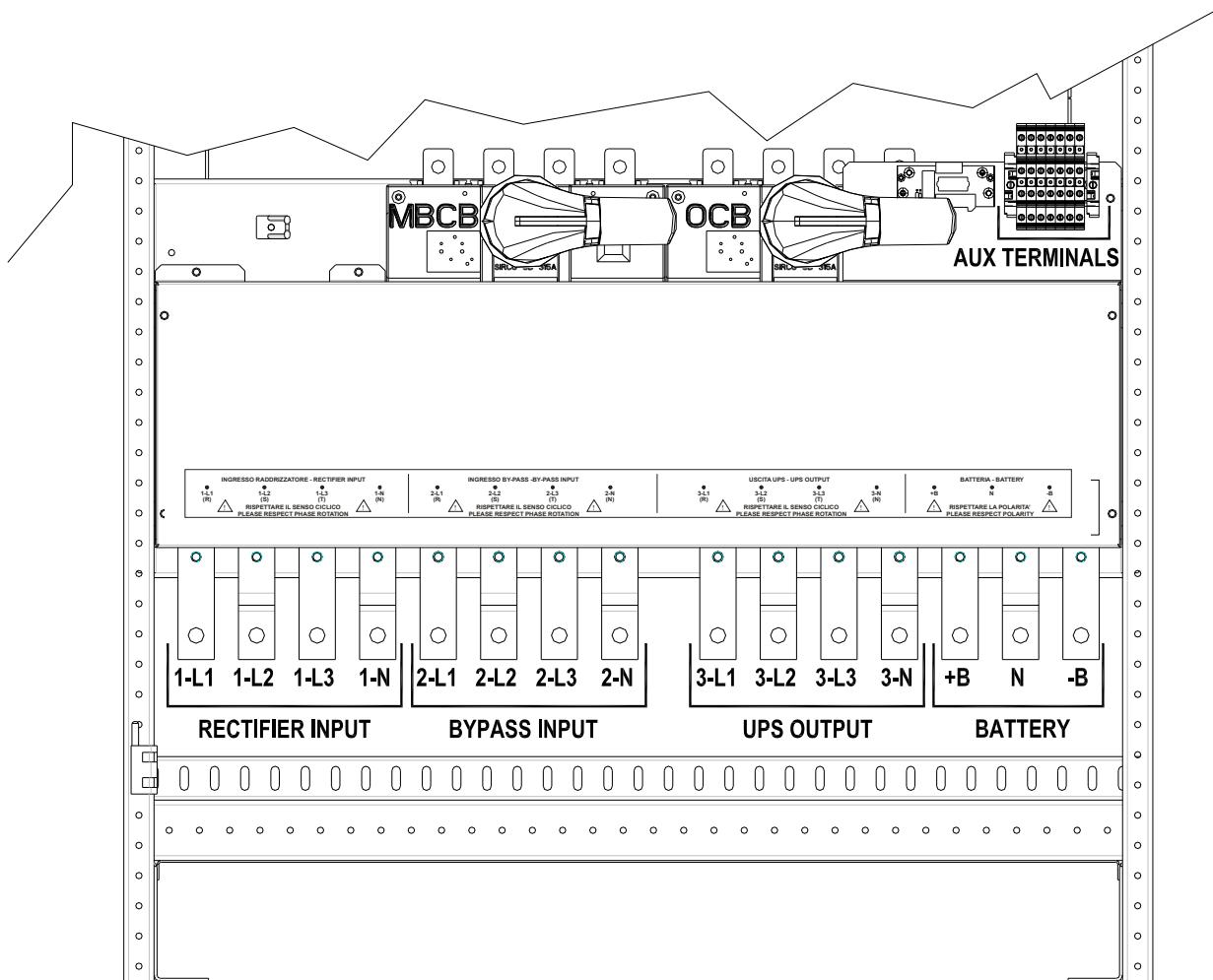
Picture 6 – Terminal board KEOR HPE 200-250 kVA
