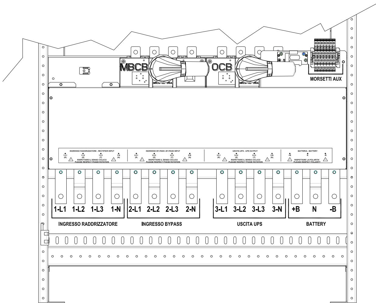
Figura 6A – Morsettiera KEOR HPE 300 kVA
