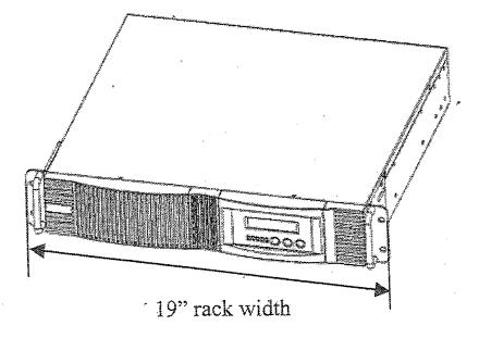
For installation the two supplied angles are to be mounted on both sides as shown on the sketch
