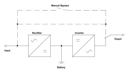
Figure 1: Block diagram "Normal operation"
