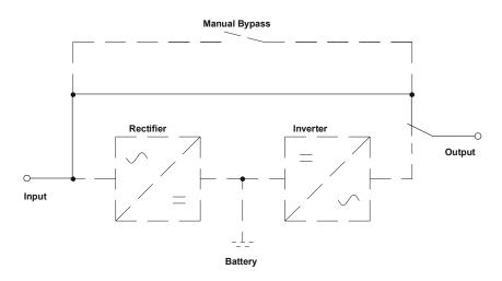
Figure 3: Block diagram "Fault in the inverter"
