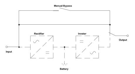
Figure 4: Block diagram "Manual bypass"
