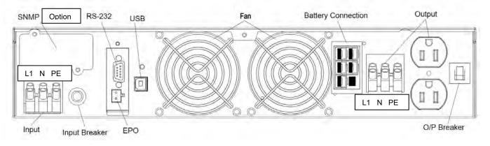
Picture 9: Rear view WÄRTSILÄ JOVYTEC PMS 3002K (115V)
