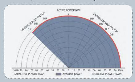
The TLE Series UPS is rated for unity output PF, but can handle a whole range of critical load power factor without UPS derating.
