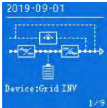
Figure4-4 Main power Inverter Output
