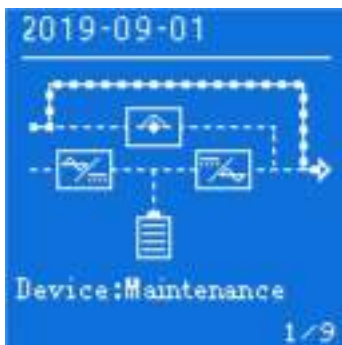
Figure4-7 Maintenance bypass output
