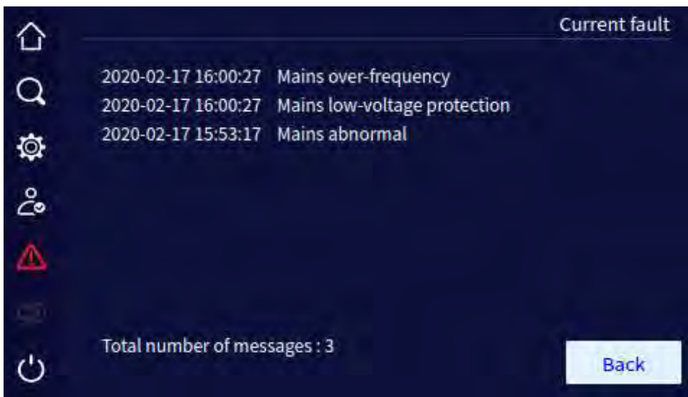
Current fault information
