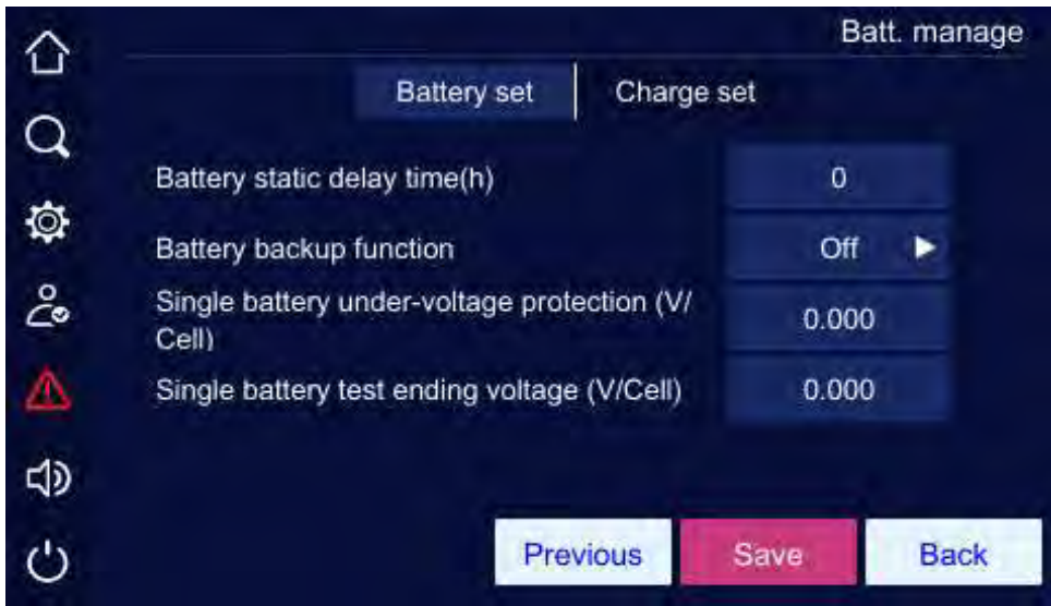
Battery set page 2 of battery management
