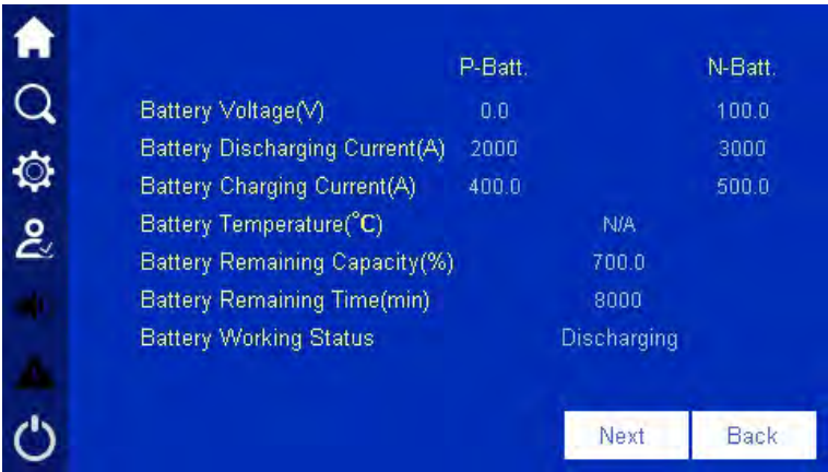
Figure4-18 Battery inversion status, battery discharge 1
