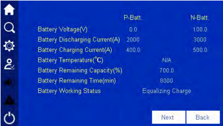
Figure4-20 Mains inversion status, battery charge
