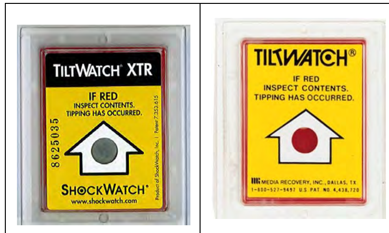
Figure 3: TiltWatch indicator: left when intact and right when tipping has occurred.
