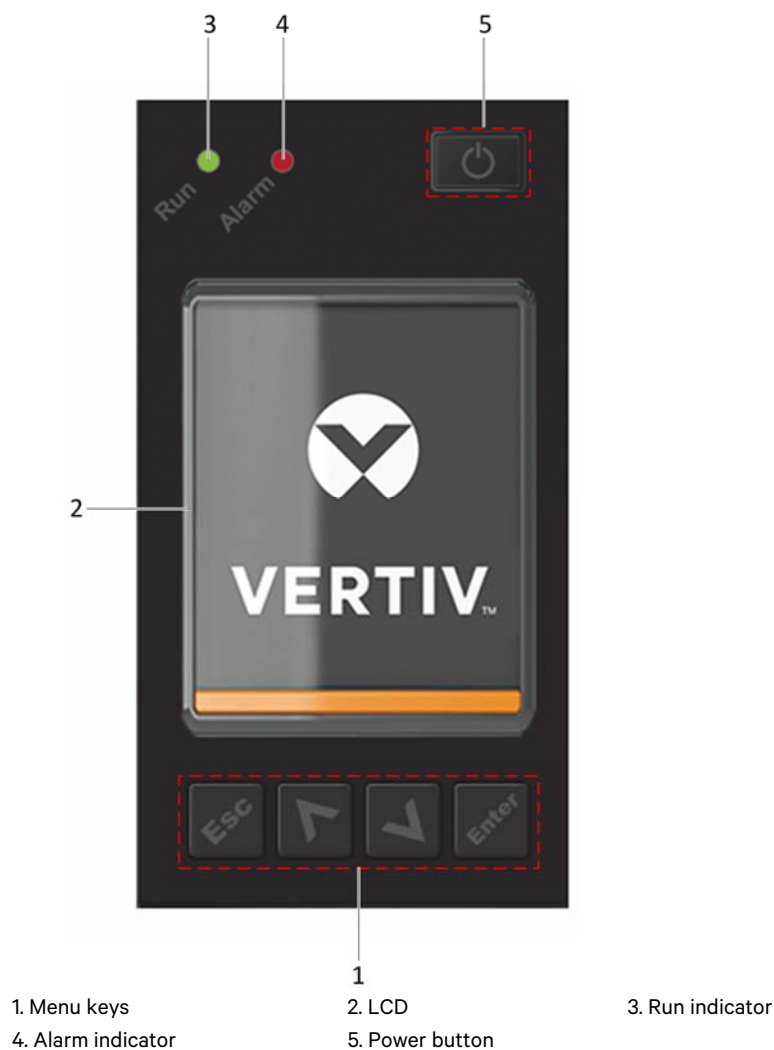
Figure 4-1 Operation and display panel
