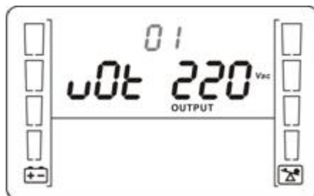
Figure 6-2 Setting the voltage level
