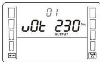
Figure 5-2 Setting the output voltage
