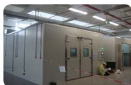
Long life test (40°C@100% load operation for 180 day)
